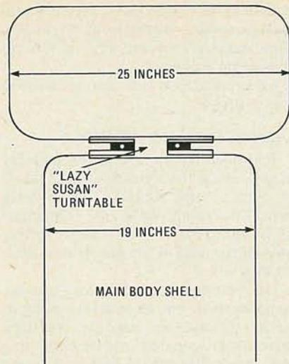
FIG. 13—THE HEAD or sensory platform rests atop the main body shell and rotates independently of the body and of the TV cameras that serves as the robot's eyes.
