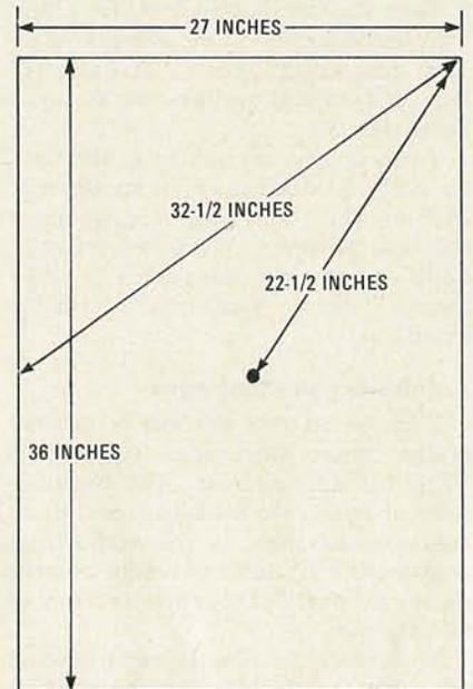
FIG. 11—DIMENSIONS and turning radius of track drive mechanism.
