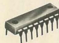
S50240. PMOS oscillator/frequency divider chip generates 13 equal-tempered notes from C<sub>3</sub> to C<sub>6</sub> to form the heart of any electronic keyboard instrument. CMOS compatible square wave outputs have 50% duty cycle for driving additional dividers or voice filters. Operates from single supply from 11 to 16 volts. 16-pin DIP.
