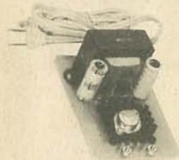
Uses LM309K. Heat sink provided. PC board construction. Provides solid 1 amp @ 5 volts. Includes components, hardware & instructions. Size:  $3\frac{1}{2}''$  x  $5''$  x  $2\frac{1}{2}''$  h
