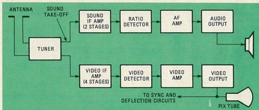
**FIG. 1—BLOCK DIAGRAM** of the IF circuit arrangement used in the Admiral 30A1 chassis, a popular 1949 model. In it, the sound take-off point was in the tuner. In many other models of this vintage, the sound take-off was at the output of the first video IF amplifier.
