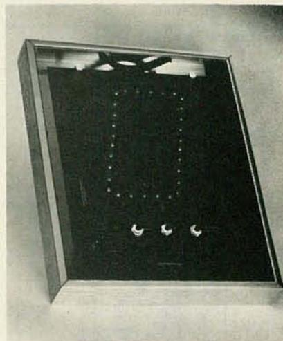
*Digital electronic clocks are no longer a novelty, except when they are designed in an unusual format. This electronic digital clock is unique in that hours and minutes are flashed sequentially in a specific pattern on a single 7-segment display nearly five inches high.*
