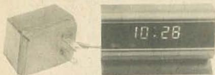
Bright .357" ht. red display. Sequential flashing colon. 12 or 24 hour operation. Black extruded aluminum case. Pressure switches for hours, minutes and hold functions. Includes all components, case and wall transformer. Size:  $3\frac{1}{4}''$  x  $1\frac{1}{4}''$
