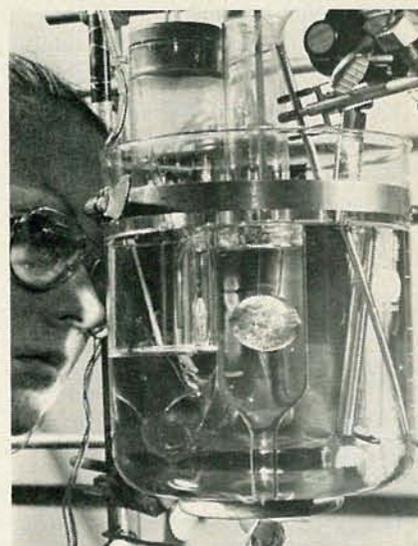
PLASTIC FIBERS STRONGER THAN STEEL are being produced by the Hughes Aircraft Co. laboratories, by vibrating a wire coil in a polymer solution at sonic frequencies and at constant temperature. The material can be seen forming inside the coil in the solution.
