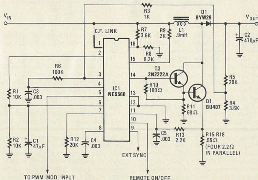
These two protective features can be investigated by looking at the output duty cycle with a scope while opening then shorting the loop.
