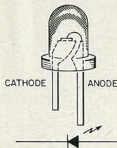
THE CATHODE IS THE SHORTER LEAD, IT IS THE BASE UPON WHICH THE LED CHIP SITS. THERE MAY BE A COLORED DOT NEXT TO THE LEAD, OR AN ABERRATION IN THE CASE DIAMETER.
