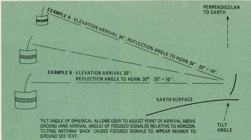
FIG. 9—TILTING THE SPHERICAL reflector surface back permits the user to adjust the angle of the reflected signals with respect to the ground.
