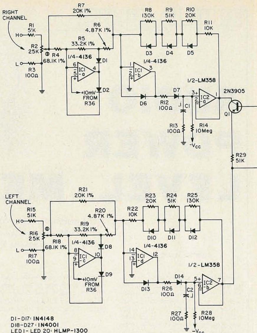
FIG. 2—COMPLETE SCHEMATIC of the LED power-level meter. The LED's in the two channels are multiplexed at a 60-Hz rate by half-sine voltages from the power transformer
