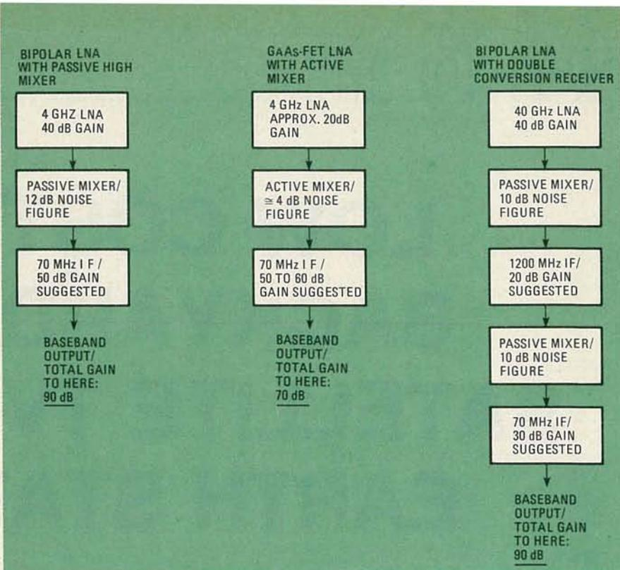
FIG. 1—GAIN REQUIREMENTS for three receiver approaches. Single-conversion receiver with bipolar LNA and passive mixer is shown in a. Single-conversion receiver with GaAs FET LNA and GaAs FET active mixer is shown in b. Double-conversion receiver with a bipolar LNA is shown in c.
