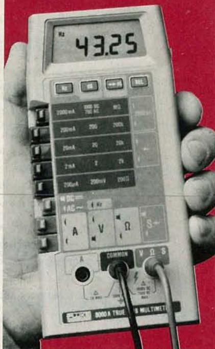
**The Fluke 8060A 4½-digit handheld multimeter.**
