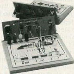
**X-TRA EDGE SOLDERLESS BREADBOARDS**. Four (4) models, each includes the Multi-use Edge Panel for mounting components which don't fit the 0.1" DIP size breadboard spacing. Transistors, SCRs, Triacs, Regulators, Heat Sinks, Switches, Lamps, Fuses, Pots, Buzzers, etc. Models include 810, 1620, 2230 and 2940 tie-points. Priced at \$16.95, \$34.95, \$49.95 and \$59.95. **CHENESKO PRODUCTS, 21 Maple St., Centereach, NY 11720**, 516-736-7977, Fax: 516-732-4650
