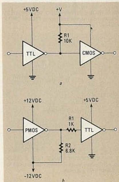
FIG. 2—INTERFACING DIFFERENT LOGIC families. Here, the methods used to interface a TTL output to a CMOS input (a) and a PMOS output to a TTL input (b) are shown.
