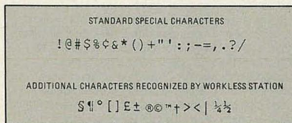
**FIG. 1—THE DEST WORKLESS STATION is an example of today's advanced OCR technology. It is capable of recognizing about 10 typefaces, which cover the majority of typestyles used commercially. Because of this, it can accept a wide variety of printed input.**
