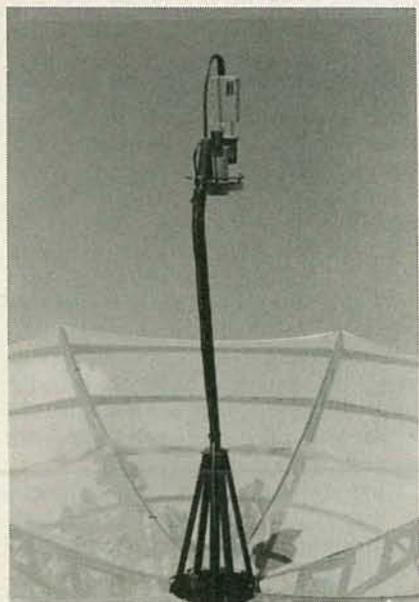
**FEED-SUPPORT ARM** places the feed and LNA (or LNB/LNC) at the focal point of the dish. The feed arm adjusts in and out to ensure precise setting for maximum signal.
