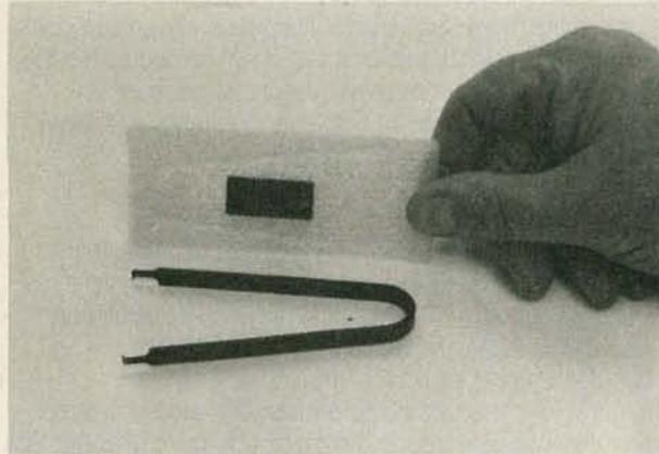
**FIG. 4—IBM's EXPANSION UNIT comes with a new BIOS ROM (on the conductive foam) and a removal tool which is used to extract the existing pre-March 1983 ROM.**
