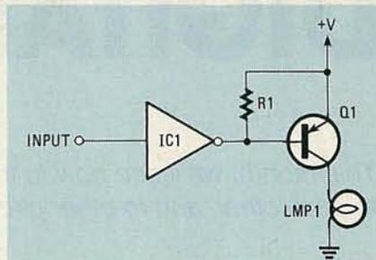
FIG. 8—A MORE COMMON METHOD of interfacing a TTL inverter with a lamp is shown here.
