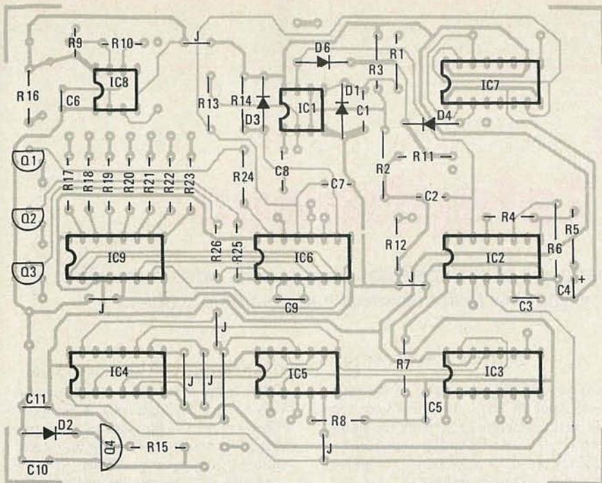
FIG. 4—PARTS PLACEMENT PATTERN for the dwell/tachometer. The PC board pattern is shown in our new "PC Service" department.
