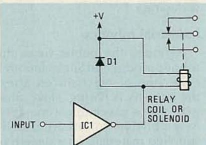
FIG. 9—AN OPEN-COLLECTOR TTL INVERTER can be used to directly control a relay or a solenoid if the device's current requirements are low enough.
