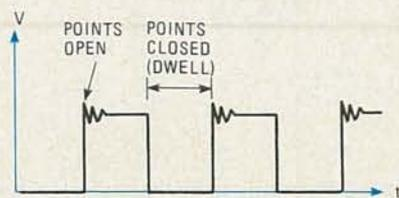
FIG. 1—TYPICAL VOLTAGE WAVEFORM of breaker points.
