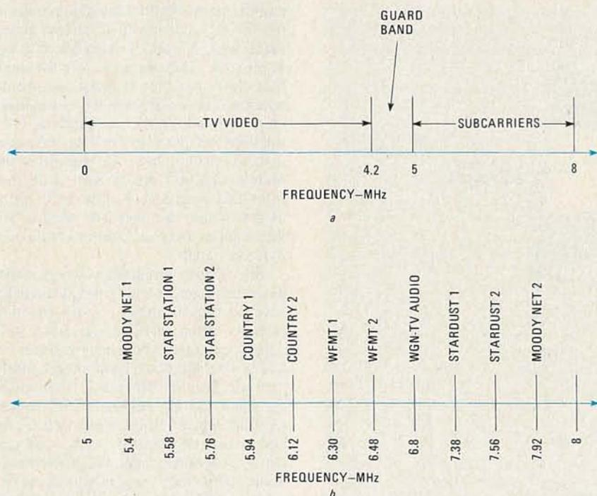
FIG. 3—A TYPICAL TRANSPONDER SIGNAL consists of the video signal, a guard band, and a number of audio subcarriers (see a). The audio subcarriers for F3R, transponder 3 (WGN) is shown in b.
