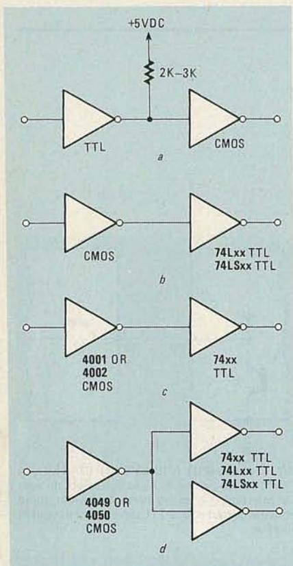
FIG. 3—MORE INTERFACING TECHNIQUES. Here, various ways of interfacing TTL and CMOS circuitry is shown.
