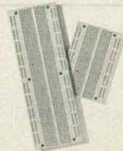
Two new solderless breadboarding sockets have been added to the Global line. The new UBS-100 is now the largest socket in the line, with 840 tie-points and the smaller UBS-500 has 430 tie-points. Each includes two rows of bus strips on each side for power and ground connections and the UBS sockets are made of the highest grade plastic material to insure maximum resistance to warping and breaking.
