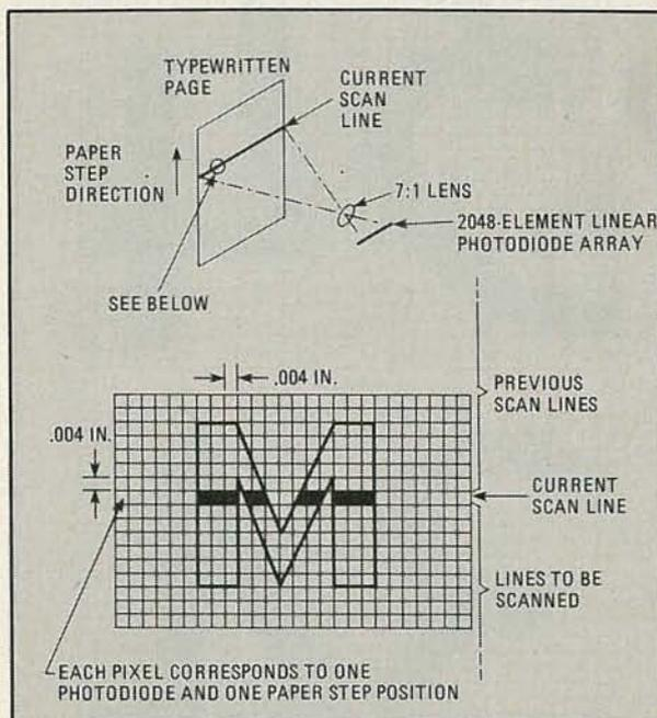
**FIG. 3—USING A 2,048-ELEMENT** linear photodiode array, an advanced OCR unit creates a series of one-pixel scan lines. The diode array detects the light. Each character occupies a 24 × 32 pixel matrix.
