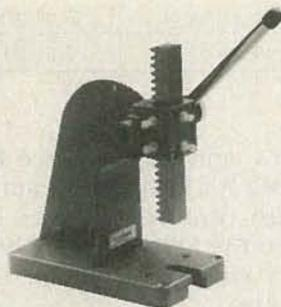
**MODEL 502 PRECISION PANAPRESS.** Less than 6 pounds, standing only 7 inches high, this hand arbor press exerts pressure up to a quarter-ton. **Panapress** is ideal for pressing bearings, sleeves or collars, forming and assembling small parts, punching, riveting, broaching, staking and dozens of other operations. Only \$65.95. See your dealer or contact: **PANAVISE PRODUCTS INC., 2850 East 29th Street, Long Beach, CA 90806.** (213) 595-7621. **CIRCLE 256 ON FREE INFORMATION CARD**
