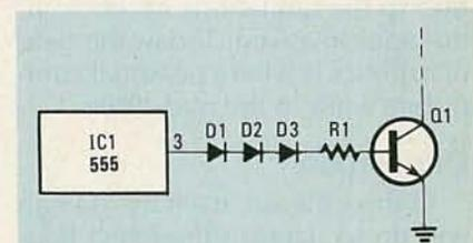
FIG. 13—A 555 TIMER CAN BE ACCIDENTALLY retriggered if noise is applied to its output terminal. To prevent that from happening, up to three diodes can be connected in series with the output, as shown.
