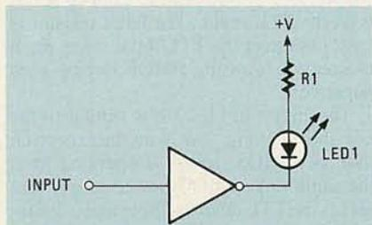
FIG. 5—THIS CIRCUIT SHOWS HOW a TTL inverter can be interfaced to an LED.
