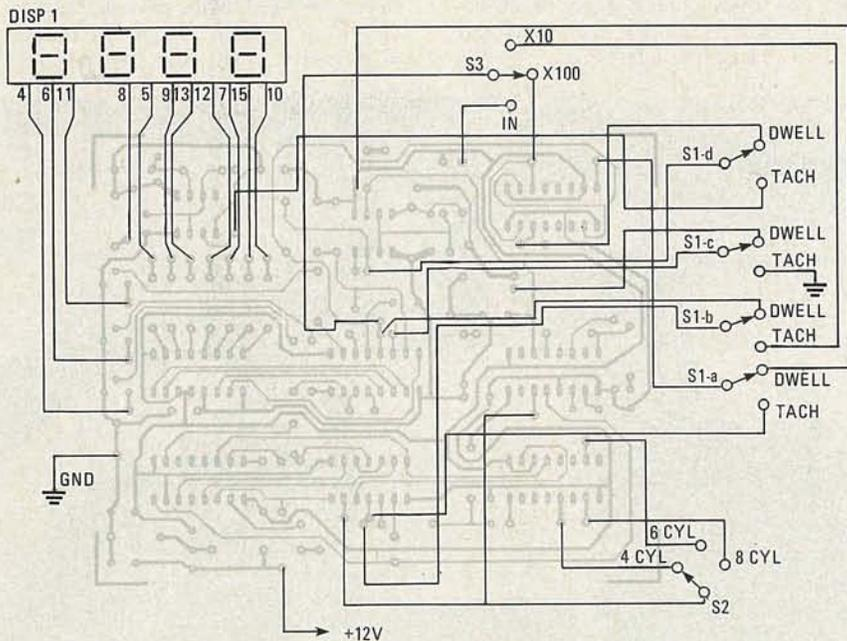
FIG. 5—THE OFF-BOARD CONNECTIONS are shown in this separate diagram.
