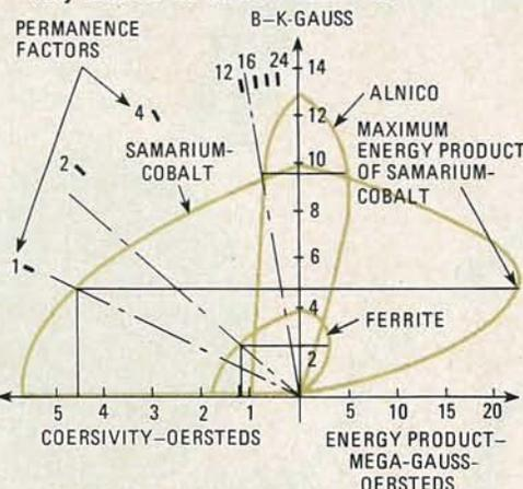
FIG. 4—THE DEMAGNETIZATION and energy-product curves for Ferrite, Alnico, and samarium-cobalt.
