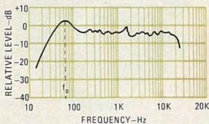
FIG. 5—TYPICAL RESPONSE CURVE for a speaker system. The frequency  $f_0$  is the minimum resonant frequency.
