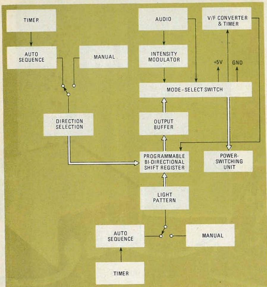
FIG. 1—BLOCK DIAGRAM of the Lumitron-4 shows the many effects available and how they are created.
