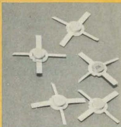
**SOLID-STATE MICROWAVE DEVICES** are vital to our efficient use of the upper end of the RF spectrum. A history of these devices, along with a description of how they function, starts on page 43.
