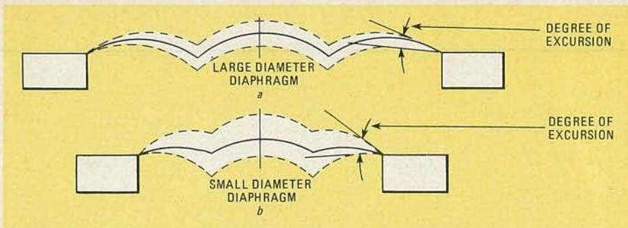
FIG. 6—VOICE-COIL LEADS ON a small-diameter driver (b) will be under greater stress than the leads on a larger-diameter driver (a).
