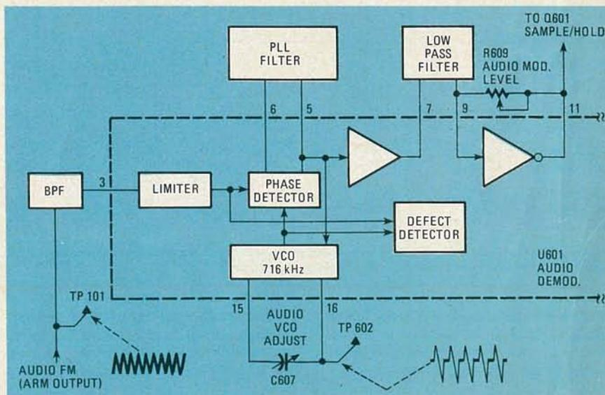
FIG. 2—AUDIO DEMODULATOR OPERATION is shown in this block diagram. Note that audio appears on a 716-kHz FM carrier. The bandpass filter rejects all other signals.
