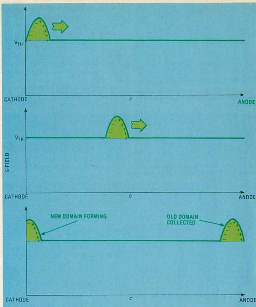
FIG. 4—WHEN the Gunn device is biased at  $V_{TH}$ , a domain builds up at the cathode end (a), drifts through the Gunn device (b), and is collected at the anode (c).
