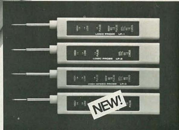
**Standard LP-1**, only \$50.00\*, with latching memory—captures pulses as fast as 50 nsec. to 10MHz, guaranteed
