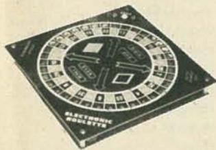
This roulette employs three CMOS IC to drive thirty-six LEDs. It includes sound effect circuit and automatic power on/off switch. Its feature can be comparable to real Roulette. It is simple in construction and easy to build.
