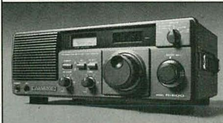
**R-600** General coverage receiver • 150 kHz-30 MHz in 30 bands • AM, CW, SSB • IF filters • noise blanker • RF attenuator • S-meter with SINPO scale • front mounted speaker • 3 antenna inputs • 100-240 VAC operation • record jack • muting terminals • digital display
